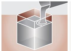
Fill the hole with the specified concrete; the foundation needs to be on the level and with a lean surface to receive the equipment; respect the instruction of the cement to dry it out. Check the correct amount with the engineer responsible for the work or installation.
