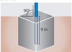
Install the board while the concrete is still fresh. Support the board with a piece of wood protecting it at 90 degrees level, and use a level for better installation. The sign needs to be at the height of 71 inches.
