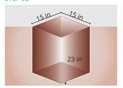
Make a hole in the following specification: 23 inches deep with 15x15 inches in diameter.
