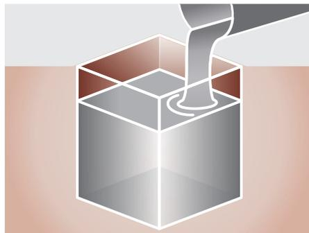
Fill the hole with the specified concrete; the foundation needs to be on the level and with a lean surface to receive the equipment; respect the instruction of the cement to dry it out. Check the correct amount with the engineer responsible for the work or installation.
